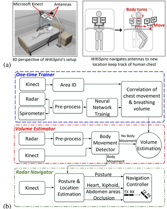
**Figure 1: *WiKiSpiro*: (a) conceptual design and (b) overview architecture.**
