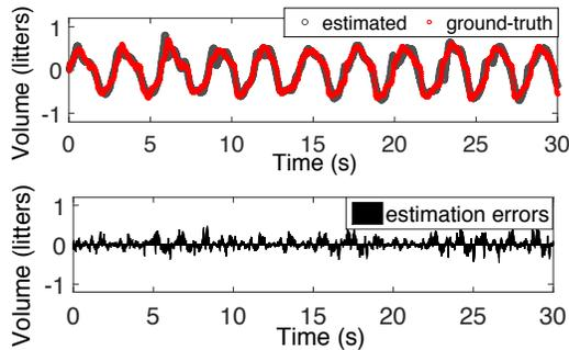
Figure 3: Breathing volume estimated by the basic *WiKiSpiro* algorithm for a stationary person.
