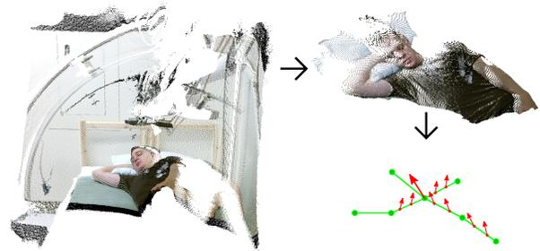
Figure 4: Depth image of the sleep environment used to identify the chest region (left). The resulting segmentation (top right) provides a basis for a reduced skeletal estimate (bottom right).
